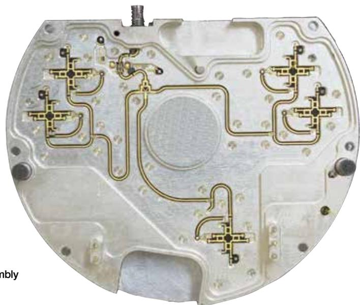
Millimeter Wave Receiver Sub Assembly
