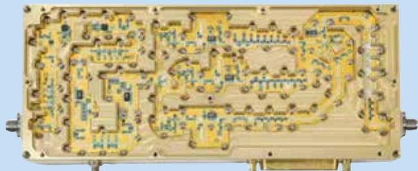
Model ACM2052 0.5 to 2 GHz Amplitude Control Module
