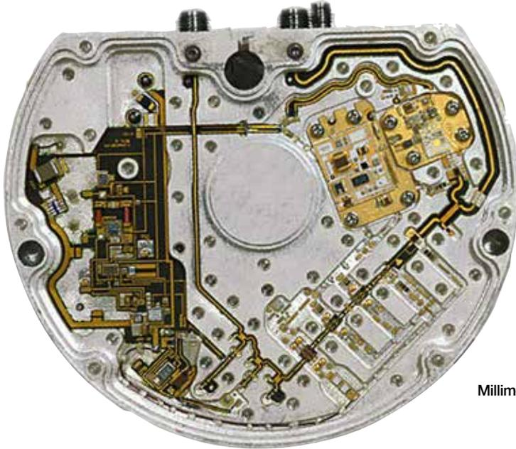
Millimeter Wave Transmitter Sub Assembly
