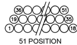
CONNECTOR MATING FACE (RECEPTACLE)
